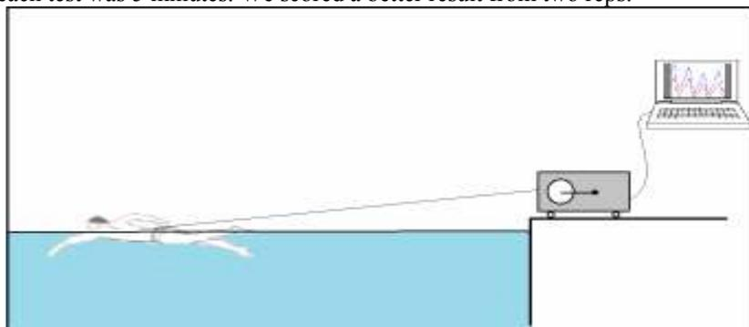
Fig. 1. Graphic representation of the performance peak test on a swimming isokinetic dynamometer at a swim speed of  $0.8 \text{ m}\cdot\text{s}^{-1}$
