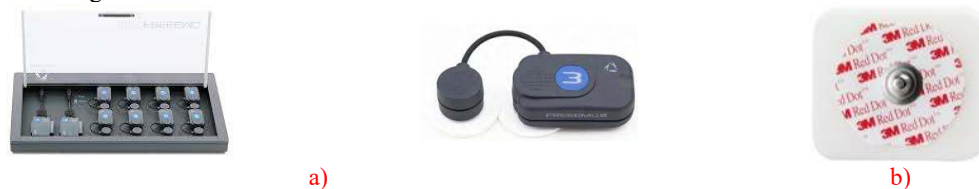
Figure 1. Equipment used for surface electromyography (sEMG) measurements: (a) reusable EMG sensors; (b) disposable Ag/AgCl-based 3M Red Dot™ electrodes
