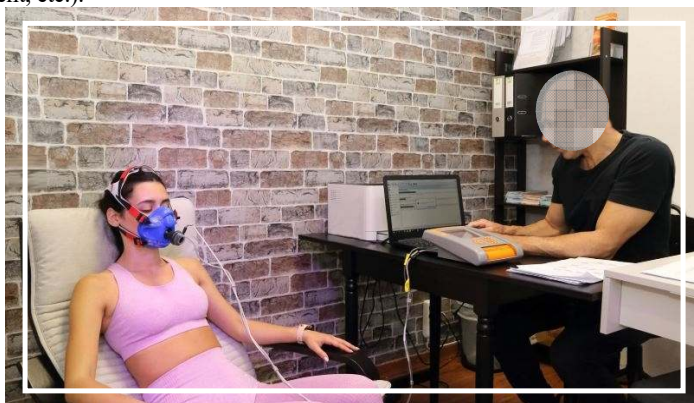
Fig. 1. Laboratory tests using the Fitmate PRO ergospirometric system
