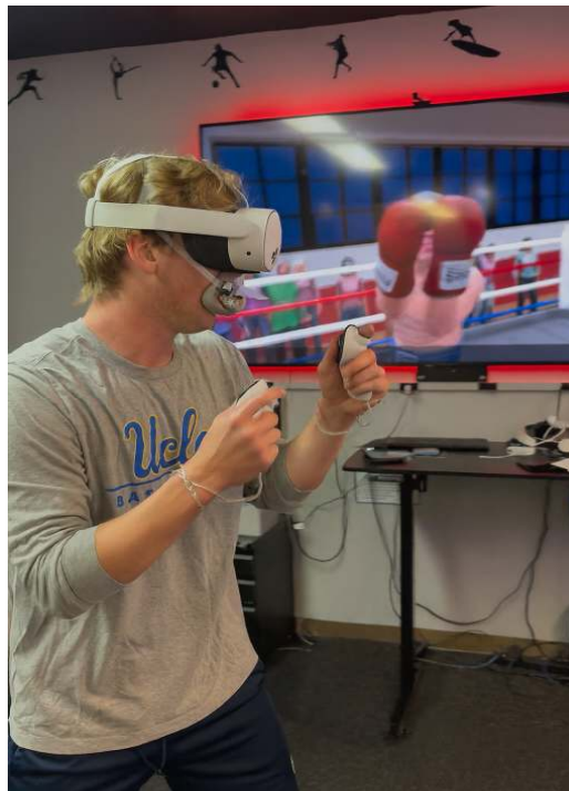
Figure I. Immersive VR exergaming gameplay showing Meta Quest 3S headset, Calibre metabolic unit and heart rate chest strap (under garment) used to assess physiological responses.
