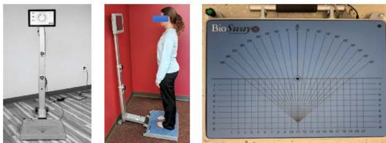
Fig 3. Biodex BioSway. The four conditions of the CTSIB-M (eyes open/closed on stable/foam surfaces) were performed on a force plate.
