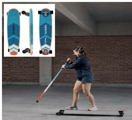
Figure 1. Complete testing setup featuring the research participant positioned on a Longboard, equipped with a handheld pole and a portable indirect calorimetry system attached to her face.
