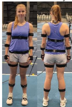
Figure 3. Placement of inertial sensors on the athlete
