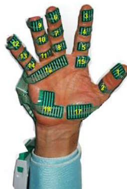
Figure 3. The Tekscan Palm pressure sensors
